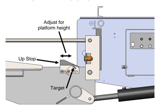
Move the sensor closer to or away from the target as required so that the sensor activates at the full up position. As with the other sensor, ensure that there no contact will be made between the target and the sensor as it will result in damage.
