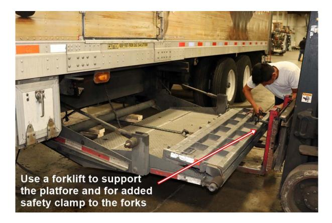
4. Before pulling the gate out to expose the rollers unclamp and disconnect the ground wire in the inner slide. Then loosen the cord grip holding the pushbutton wire and pull as much slack out as possible. (NOTE: You may need to disconnect the wiring from the terminal strip to get enough slack in the wire).
