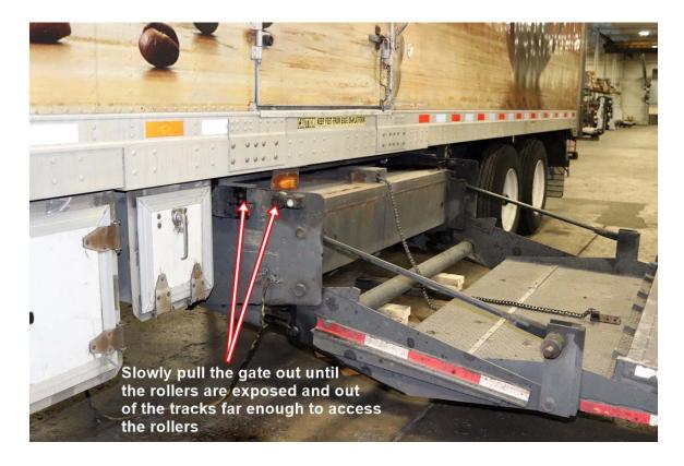
7. Remove rollers on each side and replace with new rollers.
