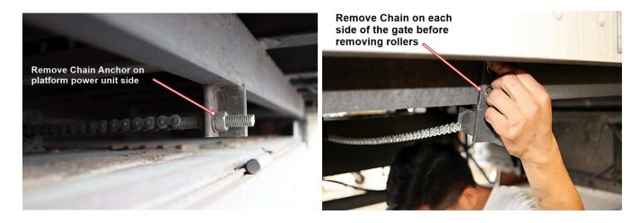
3. To remove the front rollers with the gate about 12" to 16" off the ground and all the way out use a forklift and locate the forks all the way under the platform then clamp platform to the forks for added safety.
