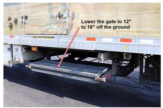
2. Disconnect the chain at both ends of the outer slide. If you are removing platform side rollers first then run the gate out before disconnecting the chain on both sides.
